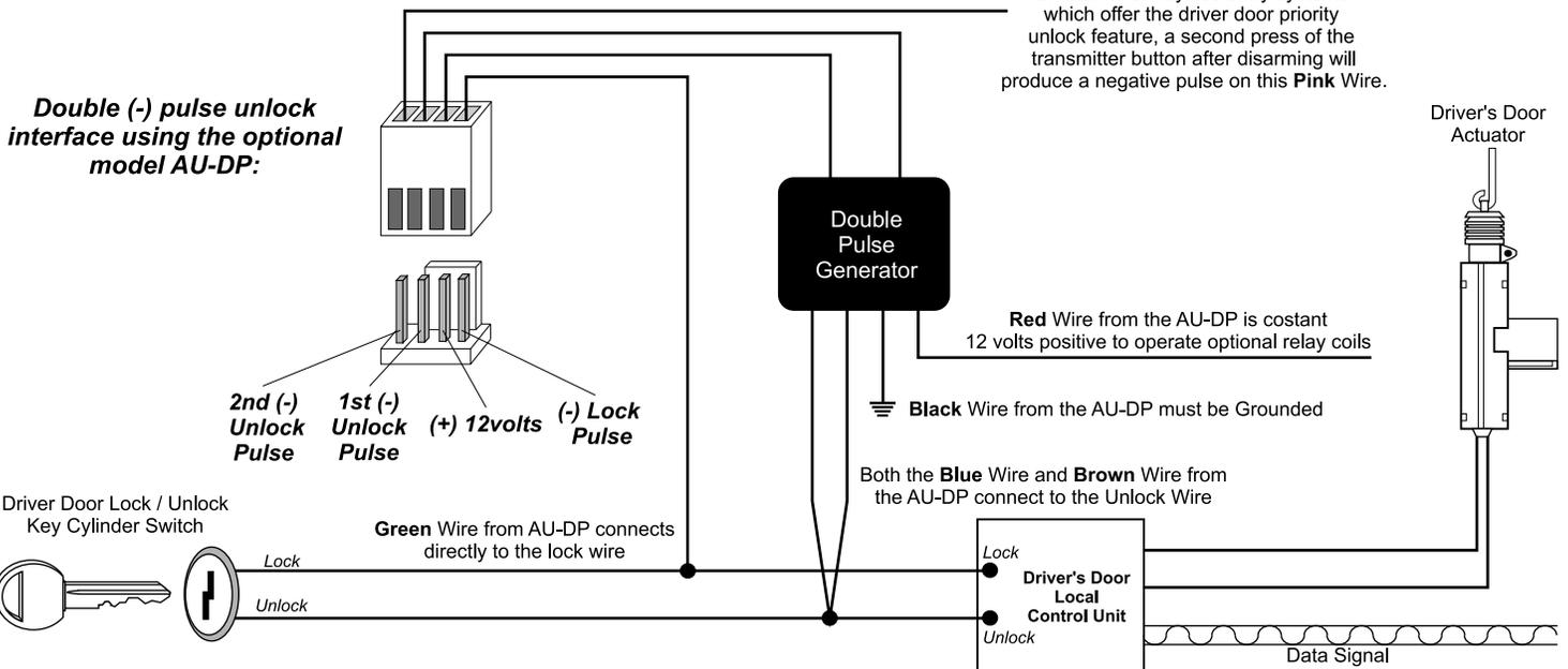
**CONNECTION:** The diagram above shows how to connect the optional model "AU-DP" to a Double Pulse type door lock system. The "AU-DP" is a pre-wired harness with a double pulse generator, which is an electronic circuit that changes a single (-) pulse to a double (-) pulse.
