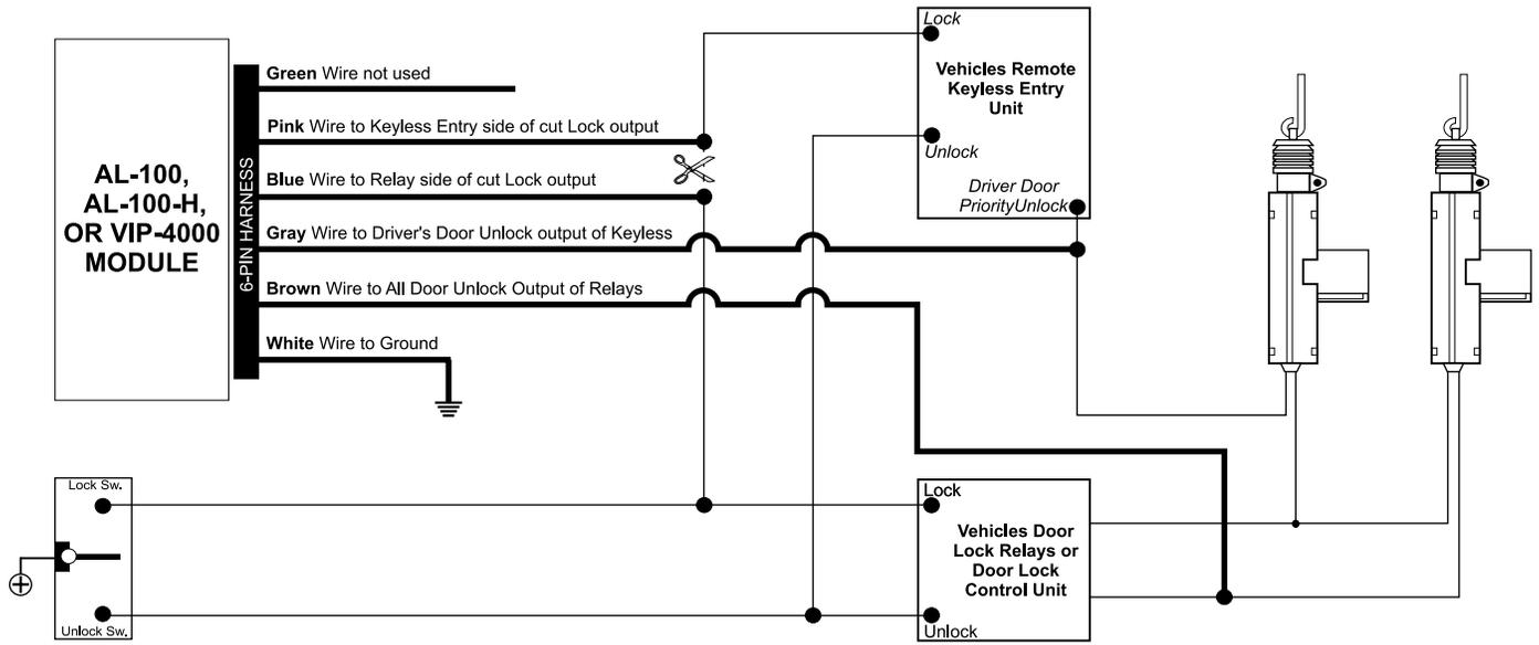
• The Type #3 Factory Keyless Entry Interface is typically used with factory keyless entry systems in which the keyless entry module is separate from the door lock relays/door lock control module. The factory keyless entry in this type of system gives positive pulse outputs to the door lock relays for all door lock and unlock and also provides a driver door priority unlock output directly to the driver's door lock actuator.
